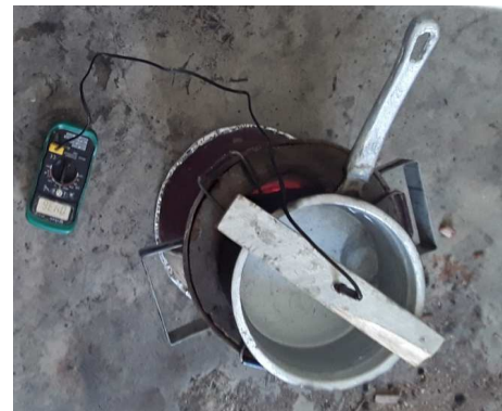
Figure 11. Test rig during WBT for ceramic jiko burning local charcoal. Digital thermal and k-type thermocouple probed into the water are shown.
